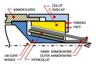
The Universal Joint (UJ) and Universal Quick Joint (UQJ) utilize a 'taper lock' termination method that ensures a cable breaking load greater than 90% of the stated parent cable breaking load. For armor cables the breaking load can range from 60kN for SA to 800kN for DA.
