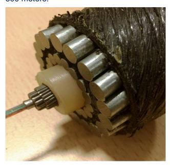
The overall cable diameters will range from 20mm for a single armor light cable (SAL) and to 65+mm for double armor heavy (DAH) cables. In extreme cases a 'rock' armor (RA) cable, comparable in diameter and weight to DA cable, is deployed but the outer layer has a very short helix length (lay length) which does not contribute tensile strength so the inner SA provides the tensile strength. This RA cable typically has a shallower deployment depth than DA.
