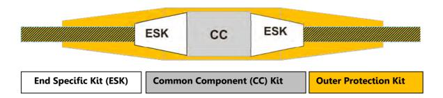
The benefits of the Universal Joint (UJ) for the repair and installation of subsea fibre optic cable systems are widely acknowledged within the Telecommunication Industry. Since its first installation in 1990 the technology has proven its reliability in-service and provides an efficient and cost effective method of connecting most types of submarine optical telecommunication cables, using a common set of equipment and standardised piece parts
